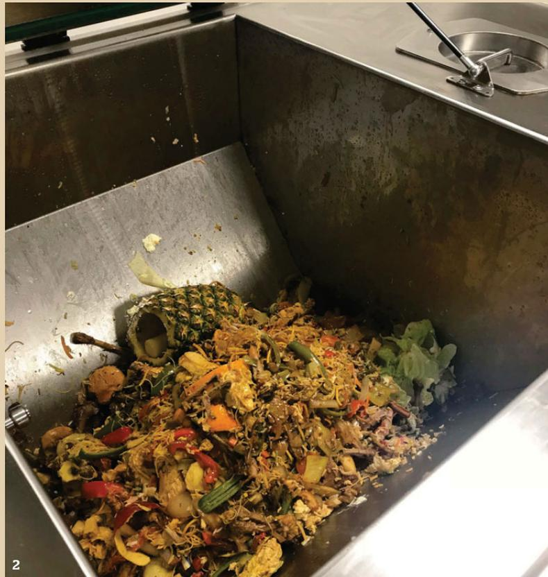
the IMC Autofeed waste system has processed 356tonnes of food waste and reduced the weight of the waste by 198tonnes. All food outlets are issued with 23-litre food caddies which are collected and replaced daily at the back door. All the caddies are weighed, and the waste is processed through the IMC Autofeed waste system where the food is disposed of into a sealed compactor and sent off for anaerobic digestion.”
